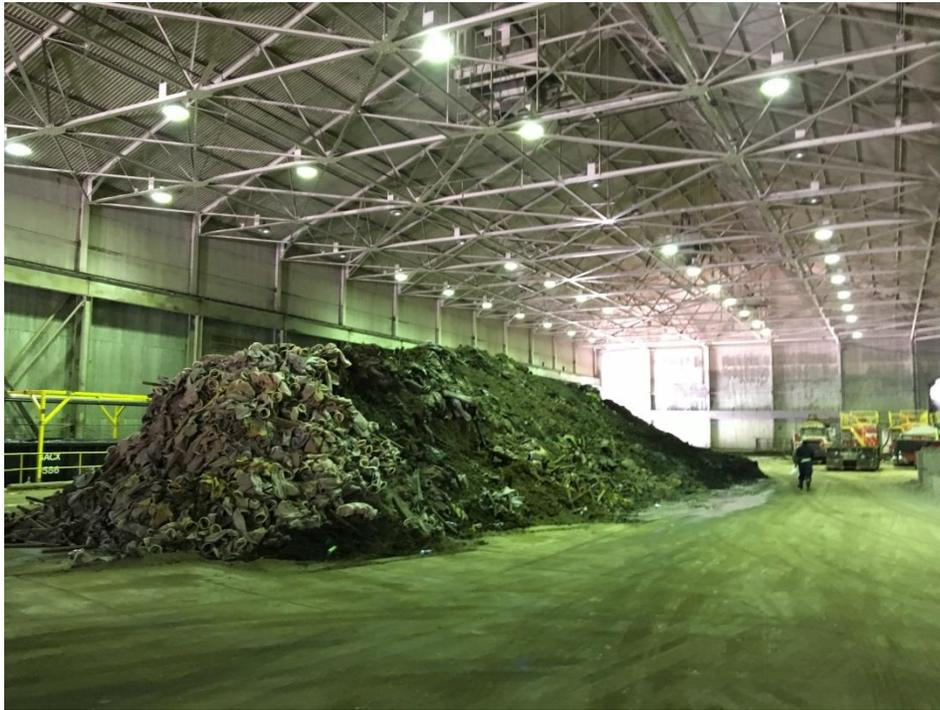
Waste pile, including filter socks, adjacent to the rail cars. Note leaching liquids from the back right edge of the pile.
