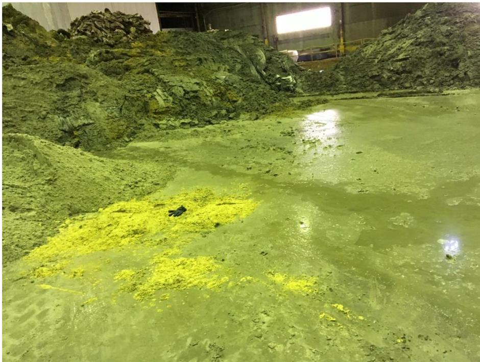
**Pile located in the right front corner of the building. Note the filter socks on the top of the pile in the left of photo. Note the leached sludge and liquid on the floor.**
